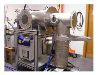
The small plasma chamber is operative since 1992 and is also a stainless steel cylinder of 0.8 meters in length and 0.4 in diameter. The baseline pressure is 10<sup>-7</sup> mbar and the working pressures when operating our small plasma thrusters are between 10<sup>-5</sup> and 10<sup>-4</sup> mbar of Argon with a gas flow around 1 sccm
